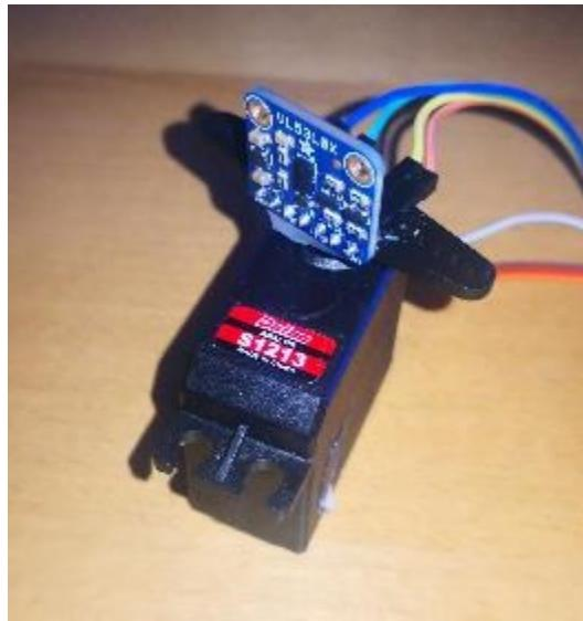
Slika 25: Arduino LIDAR
