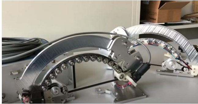
Slika 8: Arc rail moving system for plasma diagnostics (Vir: https://youtu.be/pE3-5VBnBJg?si=h_-h9xON9YHUIijz )
