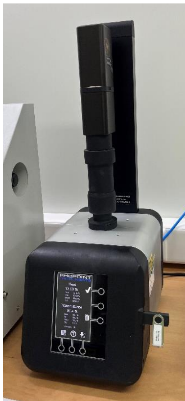
Slika 17: Merilnik motnosti NOVO – HAZE TX TRANSMISSION HAZEMETER.
