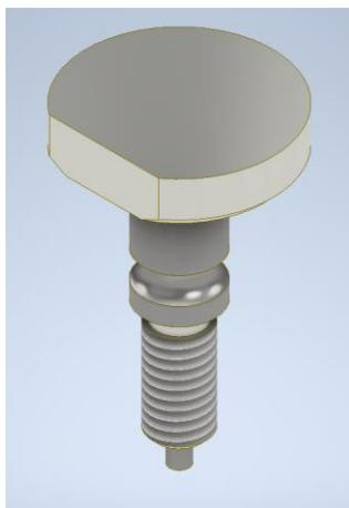
Slika 8: 3D model vijaka ventila
