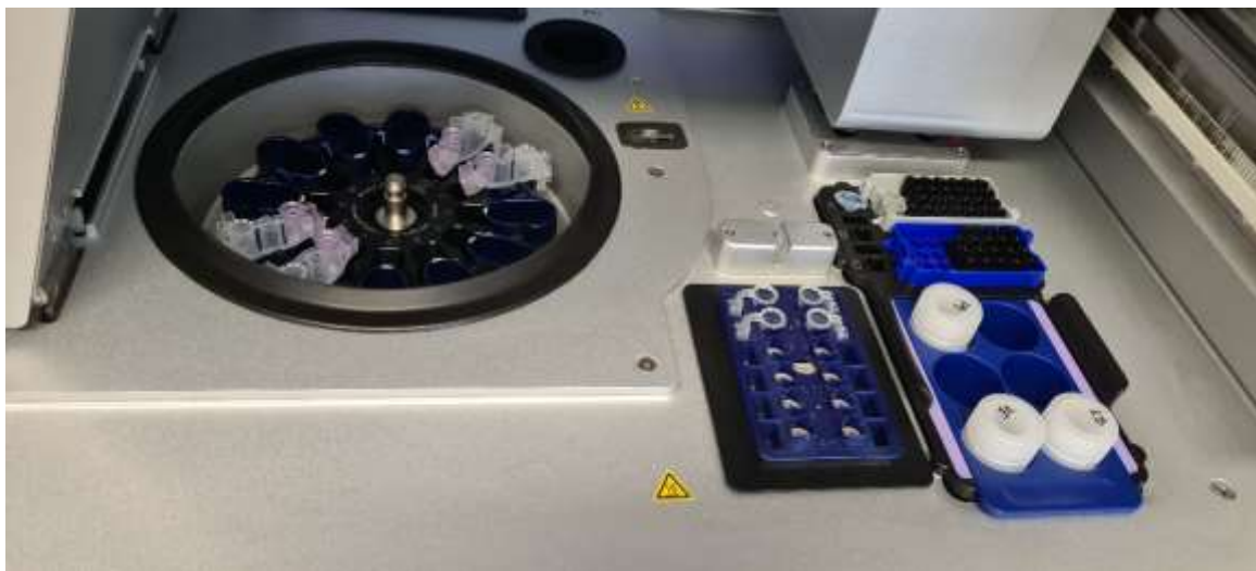
Slika 15: Aparat QIAcube in reagenti
