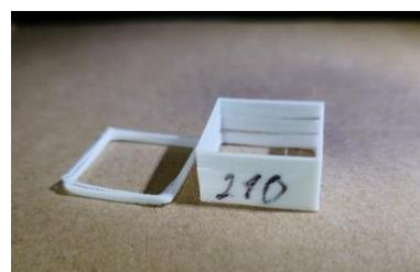
*Slika 12: Testa pri  $205^{\circ}\text{C}$  in  $210^{\circ}\text{C}$
