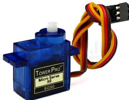
*Slika 6: SG90 servo motor.*
