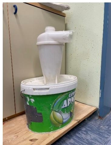
SLIKA 3. 3.17: PROTOTIP 3 S CIKLONSKIM SEPARATORJEM
