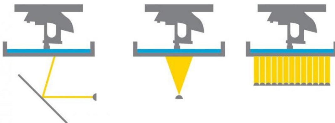
Slika 2: Prikaz delovanja stereolitografskih 3D tiskalnikov ( https://diyodemag.com/education/exploring_3d_masked_stereolithography_3d_printing )
