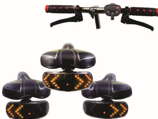
Slika 3.2: Smerniki Bicycle blinker. [10]
